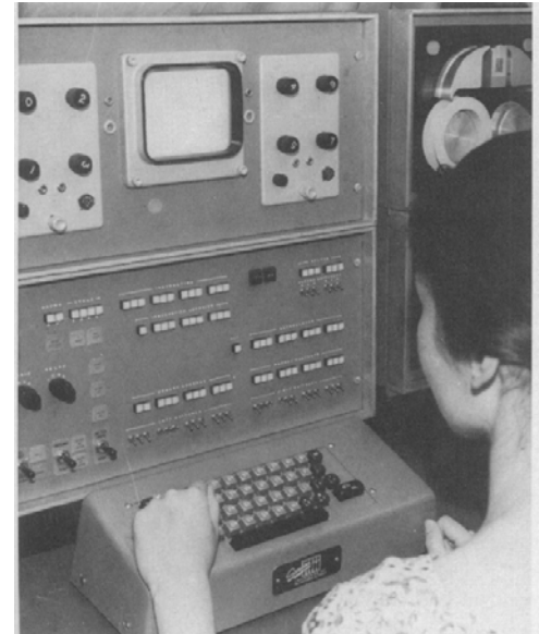
Figure 1: Site-based ePRO, 1966 style. The computer is the LINC-2, a "small high speed computer". From Slack, W. V., Hicks, G. P., Reed, C. E., & Van Cura, L. J. (1966) A computer-based medical-history system, New England Journal of Medicine , 274: 194-198
